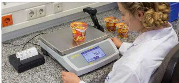
Sample testing of a pre-packaged item with an average tare value, i.e. the relative constant packaging weight is entered as a fixed value
