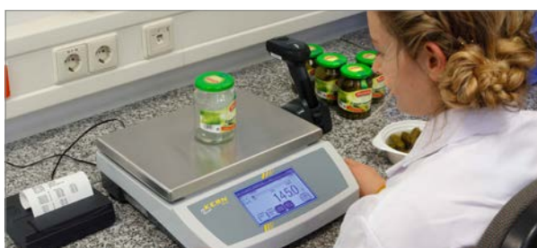
Sample testing of a pre-packaged item with fluctuating packaging weight, such as glass containers, i.e. the tare weight is entered individually for each sample.
