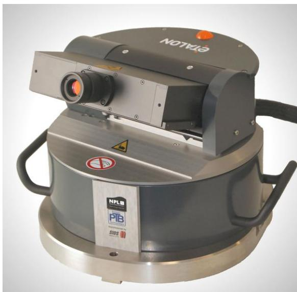
The use of the LaserTRACER improves the calibration of measuring instruments and machine tools dramatically.
