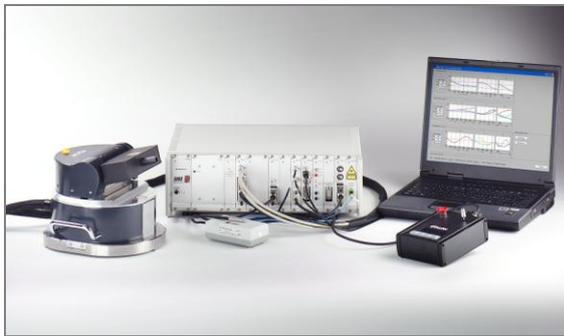
The interferometer has a resolution of 1 nm at a maximum range of 15 m. The influence of the environmental conditions is compensated by implemented temperature, pressure and humidity sensors. The laser tube is located in the external control box and guided to the LaserTRACER by a glass fibre. Therefore the thermal load is greatly reduced and a compact design can be provided. The LaserTRACER can be handled by a single operator and is applicable to machines of all working volumes.
